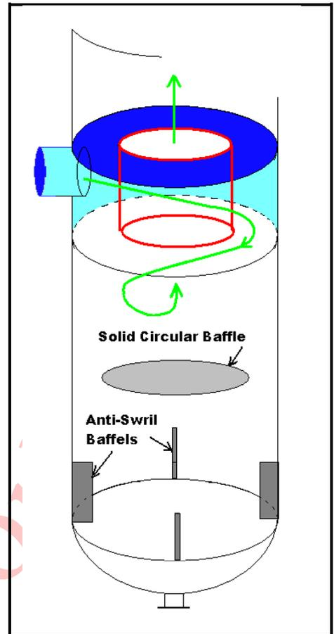
**Figure 10** – Tangential Inlet with Annular Ring
