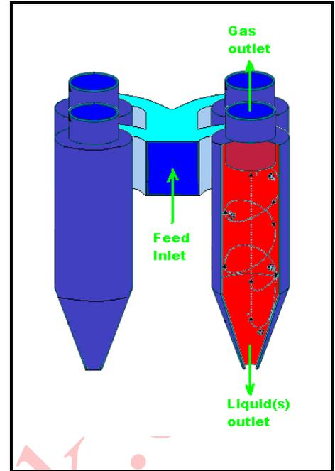
**Figure 5– Multi Cyclone Inlet Device**
