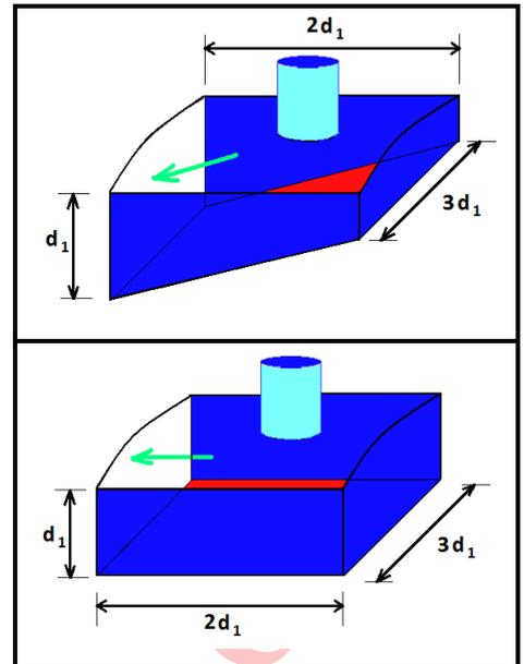
Figure 6 - Deflector Baffle Dimensions
