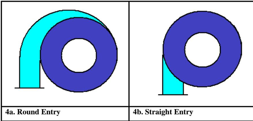
**Figure 4 - Tangential Inlet Entry Arrangements**
