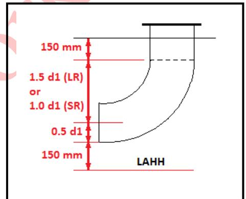
Figure 7 – Inlet Elbow Dimensions
