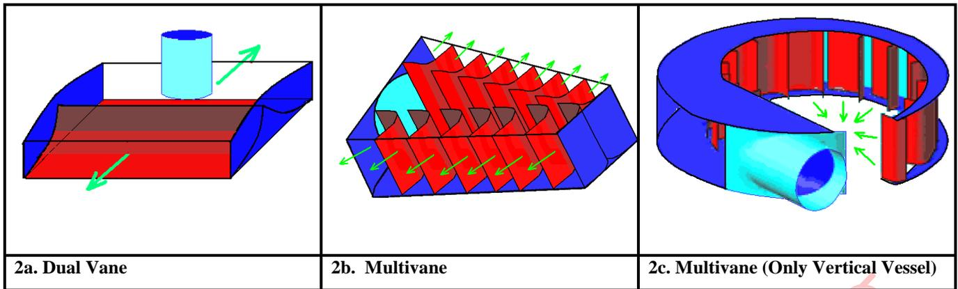
**Figure 2** – The Different Types of Vane Inlet Devices
