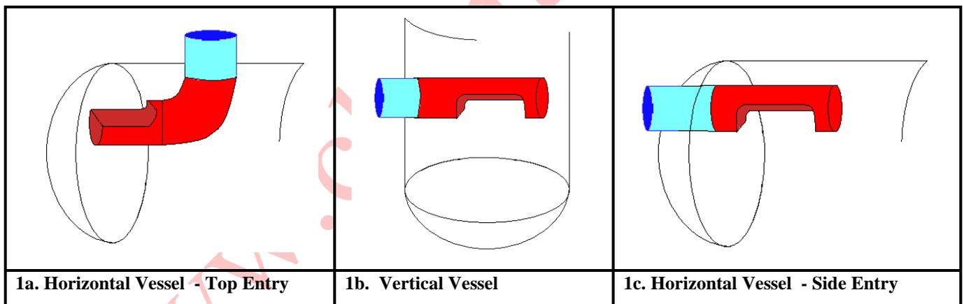
**Figure 1** – Half Open Pipe Installation Configuration in Horizontal and Vertical Vessels
