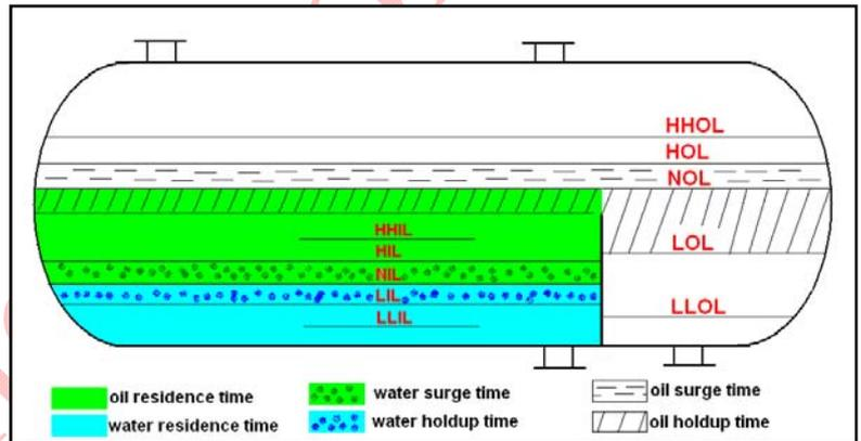
**Figure 3** – Time Definition for Submerged Weir Configuration
