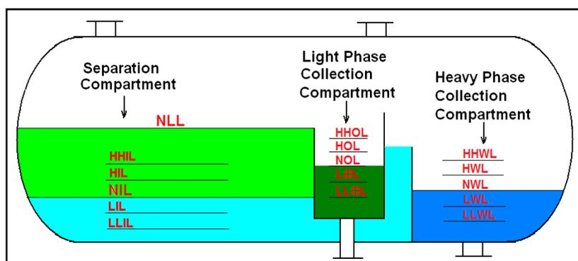
Figure 1 – Three Phase Separator Compartments and Levels
