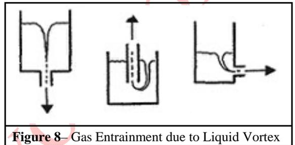
**Figure 8** – Gas Entrainment due to Liquid Vortex
