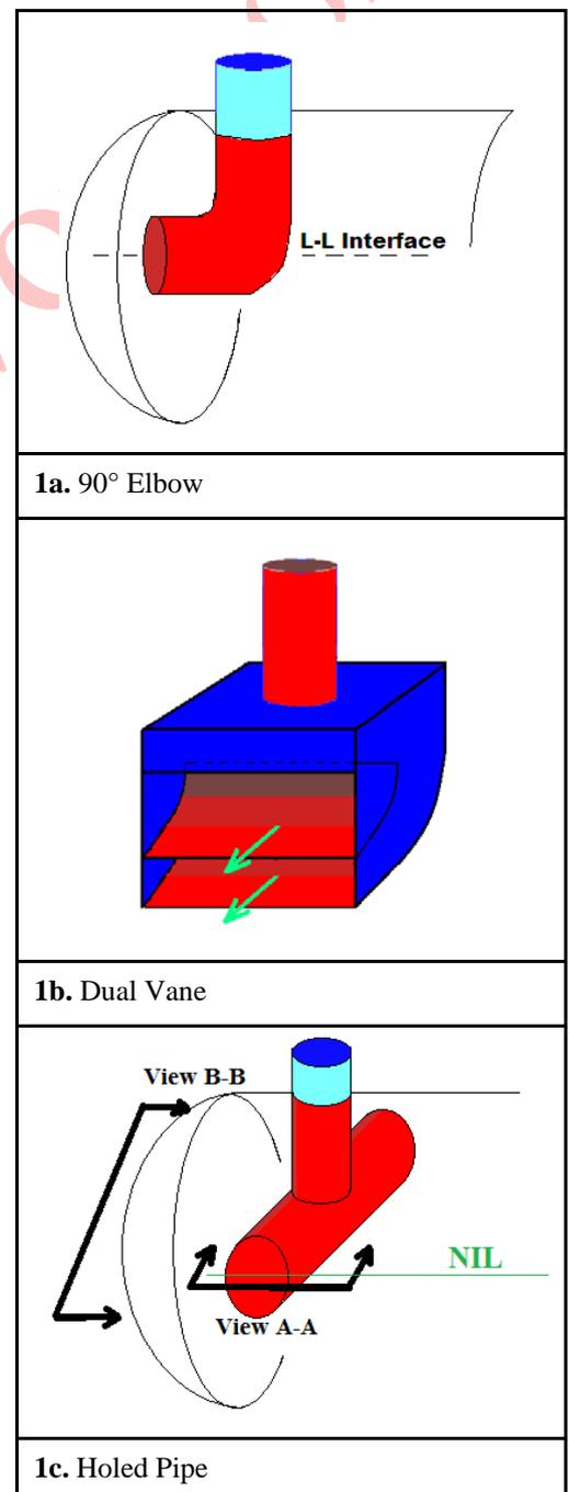
The following section provides some guidelines on the sizing of holed tee distributor:
