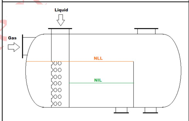
Figure 3 - Perorated Pipe Inlet Device for Three Phase Separator
