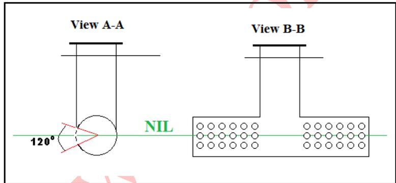
Figure 2 - Holed Tee Distributor Details
