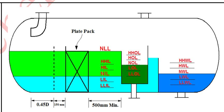
**Figure 6 – Overall Configuration of Three Phase Separator with Plate Pack**
