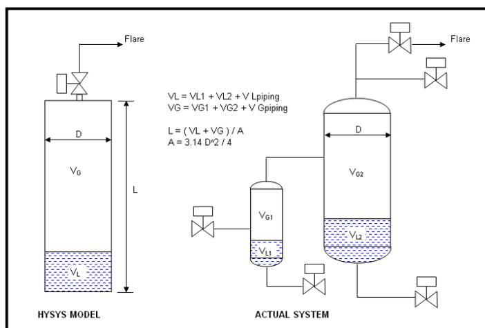
Figure 1 – Schematic of Hysys model vs. actual system
