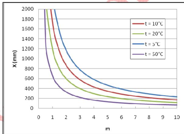
Figure 5 – Piping spool length when T<sub>b</sub> is -46°C
