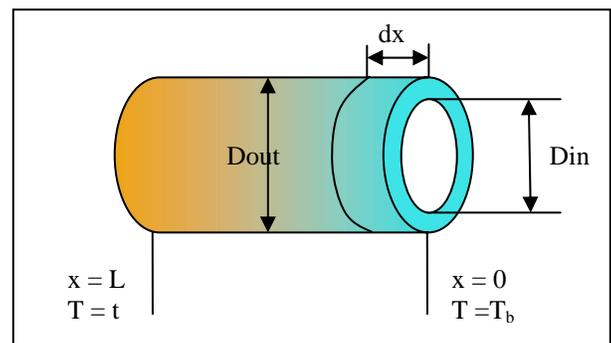
Figure 2 – Equation (4) boundary conditions
