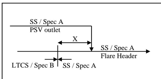
Figure 6 – location of material/piping break
