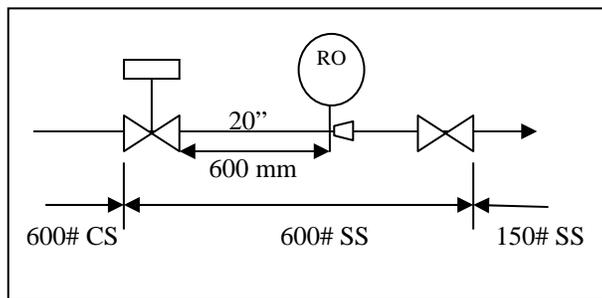
Figure 3 – BDV spec break arrangement
