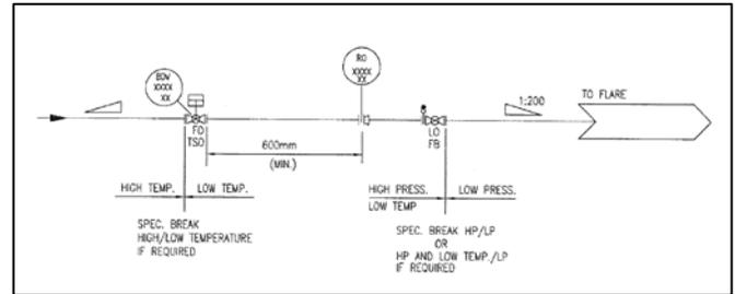
Figure 1– Automatic depressurization valve arrangement
