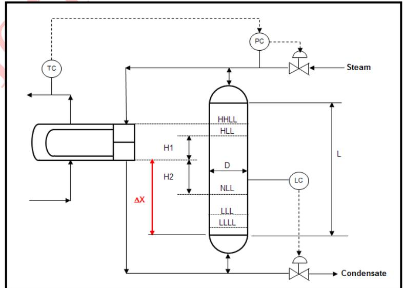
Figure 2 – Process Control via Steam Temperature Manipulation
