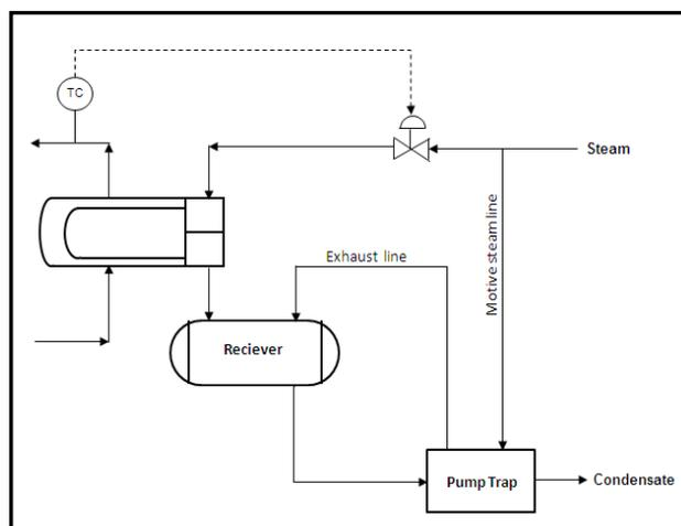
Figure 4 – Pump Trap Piping Arrangement
