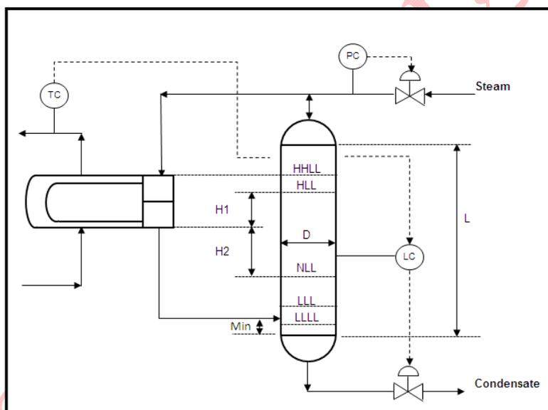
Figure 3 - Process Control via Heat Transfer Area Manipulation
