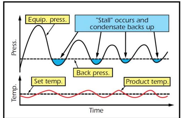
Figure 1 – Effect of Heat Exchanger Flooding
