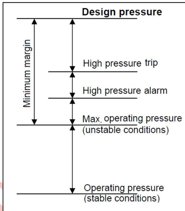
**Figure 1** – Margins between operating and design pressure
