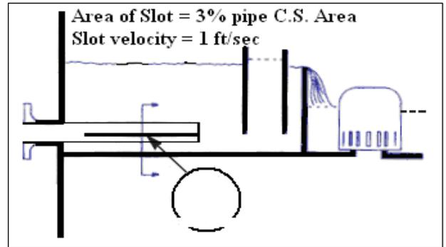
Figure 2b – Slotted pipe vortex breaker
