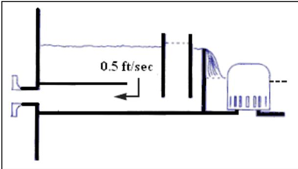
Figure 2a – Plate extension vortex breaker
