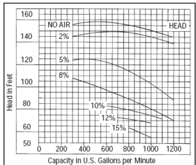
Figure 1 – The effect of air on head water pump
