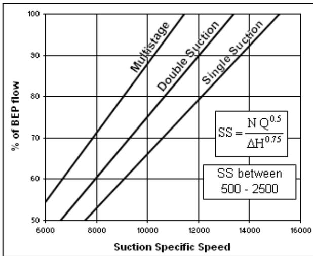
**Figure 4a** – Suction recirculation starting flow at low SS
