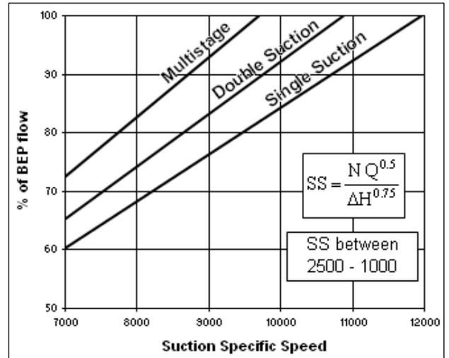
**Figure 4b** – Suction recirculation starting flow at high SS
